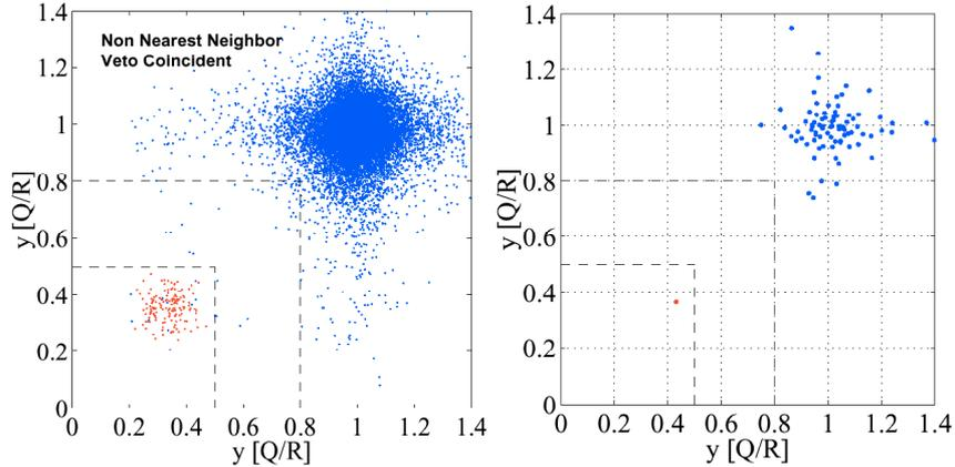
Figure 2. Multiple scattered events between non-nearest neighbouring detectors in the stack of Tower 1 run in SUF Run 21. (Left) Veto Coincident, MC predicts that 39% of all multiply scattered neutrons should be non-nearest neighbour,  $44 \pm 3\%$  observed in data, negligible beta-like contamination is evident. (Right) Veto Anti-coincident, MC predicts 2 neutron candidates, one observed. No beta-like contamination is apparent.
