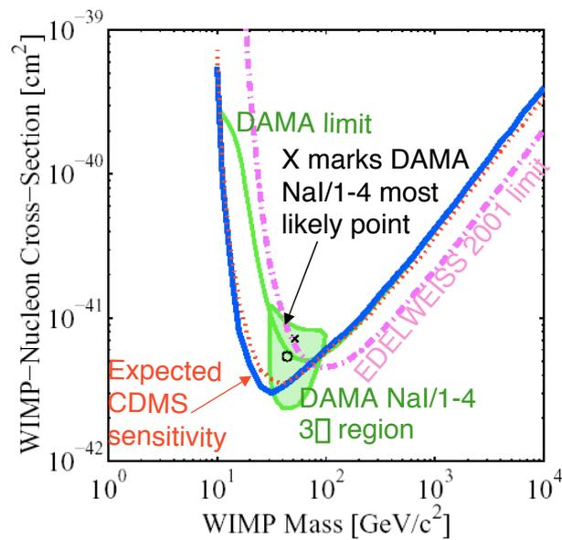
Figure 1. Exclusion limit on WIMP-nucleon cross-section from SUF Run 19, including larger fiducial volume<sup>2</sup>. The solid line is the CDMS I result, including neutron subtraction. The dotted line is the CDMS I expected sensitivity. The dot-dashed line is the EDELWEISS 2001 limit, which has since been exceeded by their 2002 limit<sup>3</sup> (not shown). For further details and relevance of the DAMA results shown see Refs. 1 and 2.
