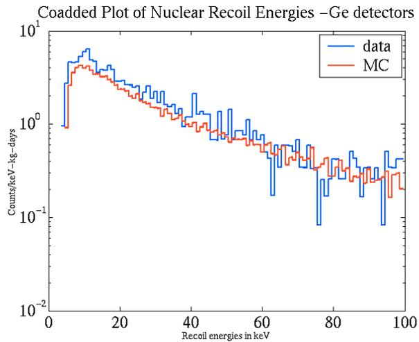
Figure 3. Comparison of muon-coincident (internal neutrons) nuclear recoil energy spectrum from Monte Carlo simulations including the same cuts as present in the data from the Ge ZIP detectors operated in SUF Run 21.
