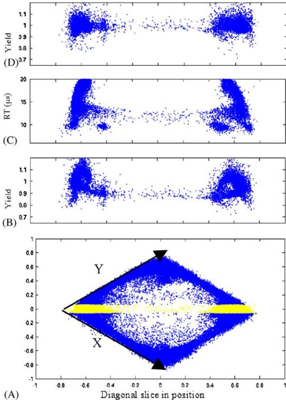
Fig. 2. All plots share the same  $x$ -axis, i.e. position based on phonon energy partition. (A) Phonon energy partition plot, showing events selected from the diagonal (light dots) for plotting in the other three subplots. (B) Charge yield, showing outer events give higher yield. (C) Rise time shows the same behavior toward the outer parts of the detector. (D) Charge yield after the correction by the method described in the text.
