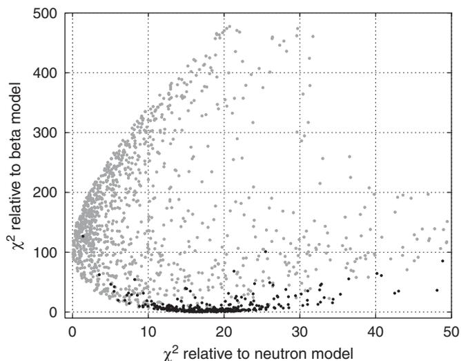
Fig. 1. Chi-squared discrimination. On the  $x$ -axis is  $\chi^2$  relative to the neutron model, and on the  $y$ -axis is  $\chi^2$  relative to the surface contaminant (beta) model for  $^{133}\text{Ba}$  surface scatters (dark) and  $^{252}\text{Cf}$  neutrons (light).
